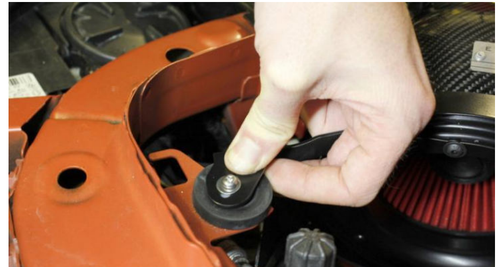
42. Push the mount all the way into the grommet. (Photo shown without the duct)
