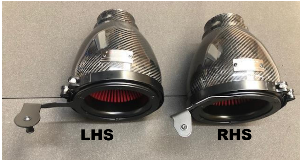
30. Identify the left and right side intakes. The left side has the mounting bracket secured around the bottom of the opening. The right side has it secure around the top as shown. The brackets are also a different shape.
