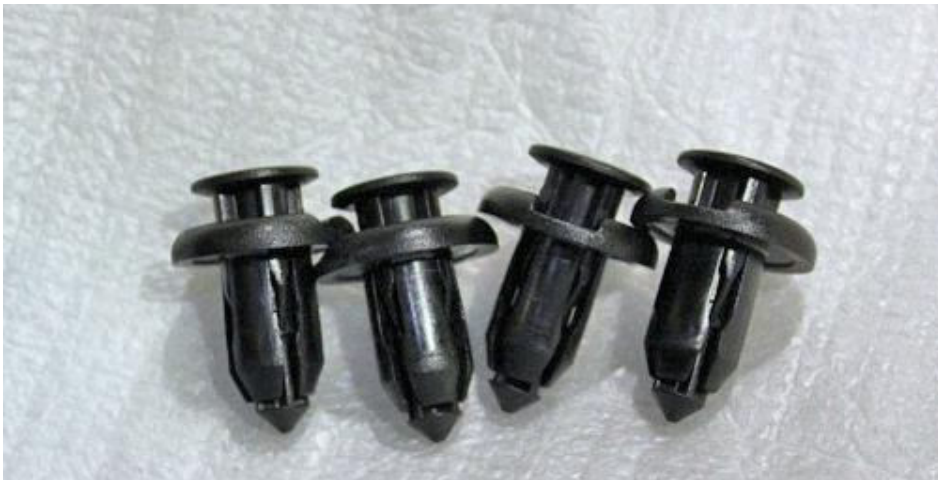
19. We will now install the ducts which direct cold air into the intakes. These 4 push rivets will be used for the installation.
