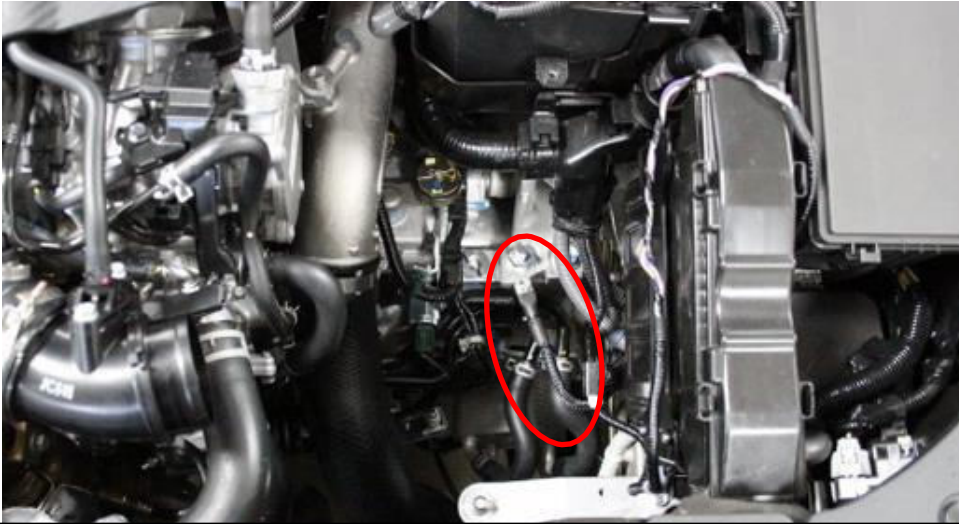
5. Locate the earth strap as shown.
