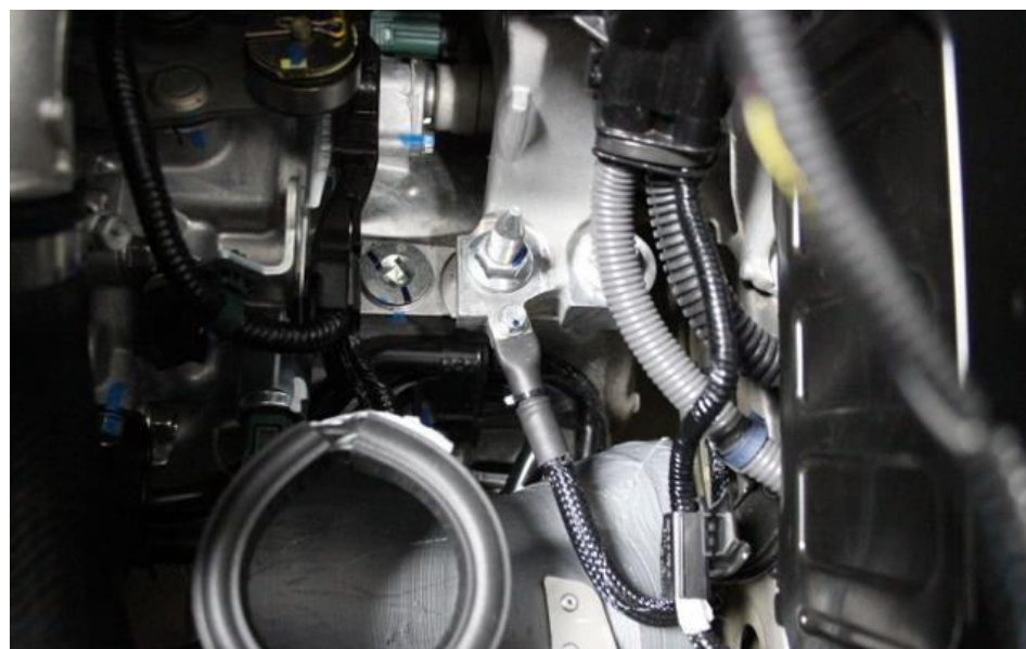
14. Secure the earth strap back into place with the OEM bolt previously removed.
