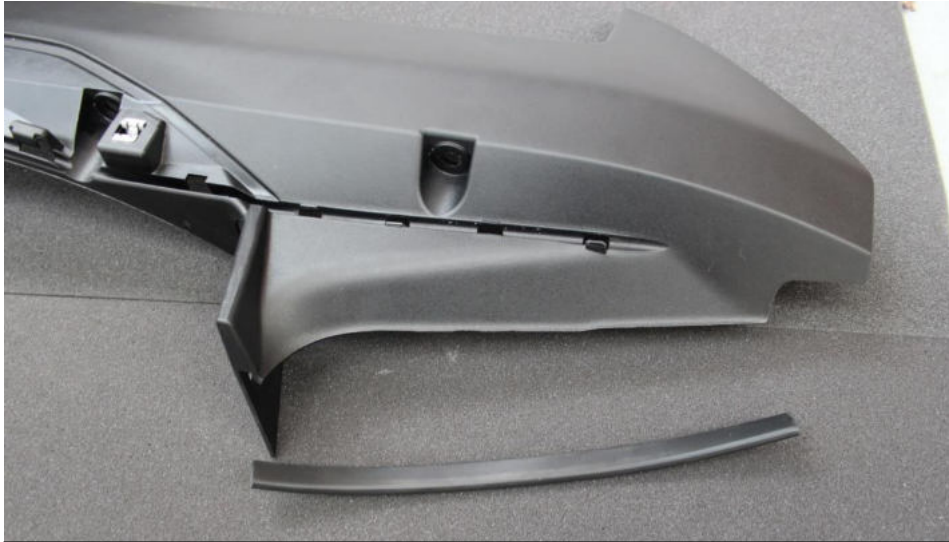
33. Take the supplied rubber strips and push them onto each side of the front plastic trim removed from step 4. See next photo.
