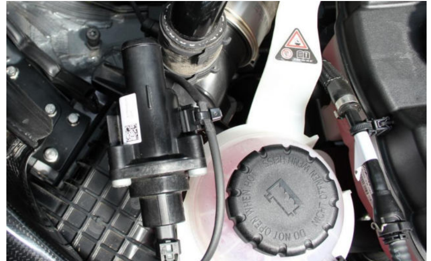
6. Remove the rubber hose completely and retain the spring clamps.
