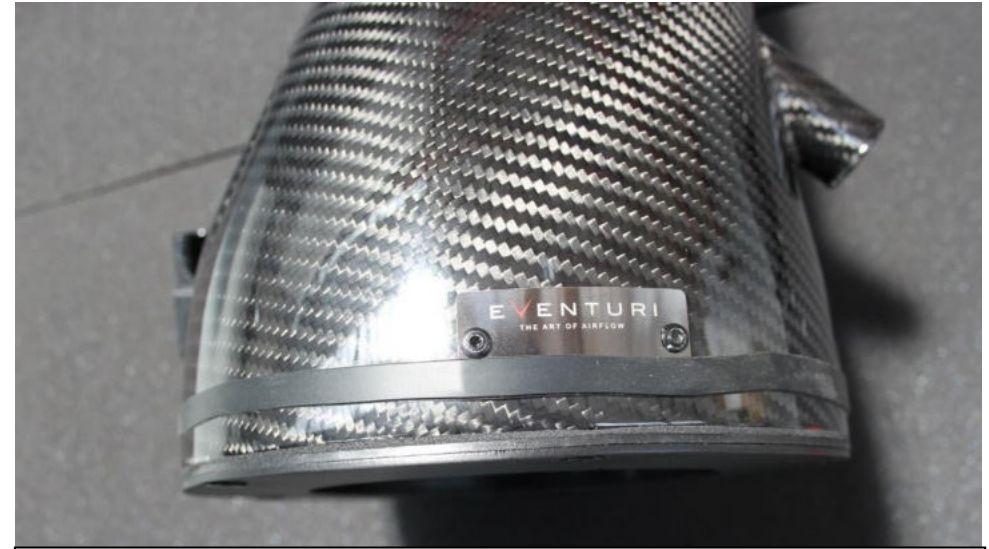
22. Take the LHS Housing and pull the black band back as shown – otherwise it will get caught on the duct during installation and come off.
