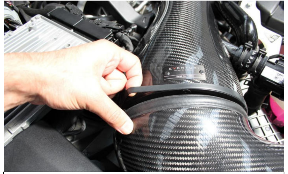
28. Move the band back into place so that it covers the joint between the filter and the carbon housing.
