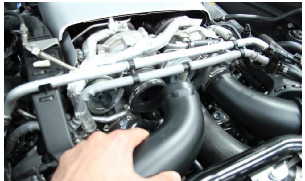
8. Loosen and remove the tube to the Turbo inlet.
