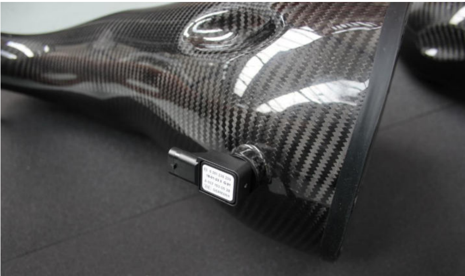
15. Insert the sensors into the sides of the housings - push them in and turn 90 degrees to secure.
