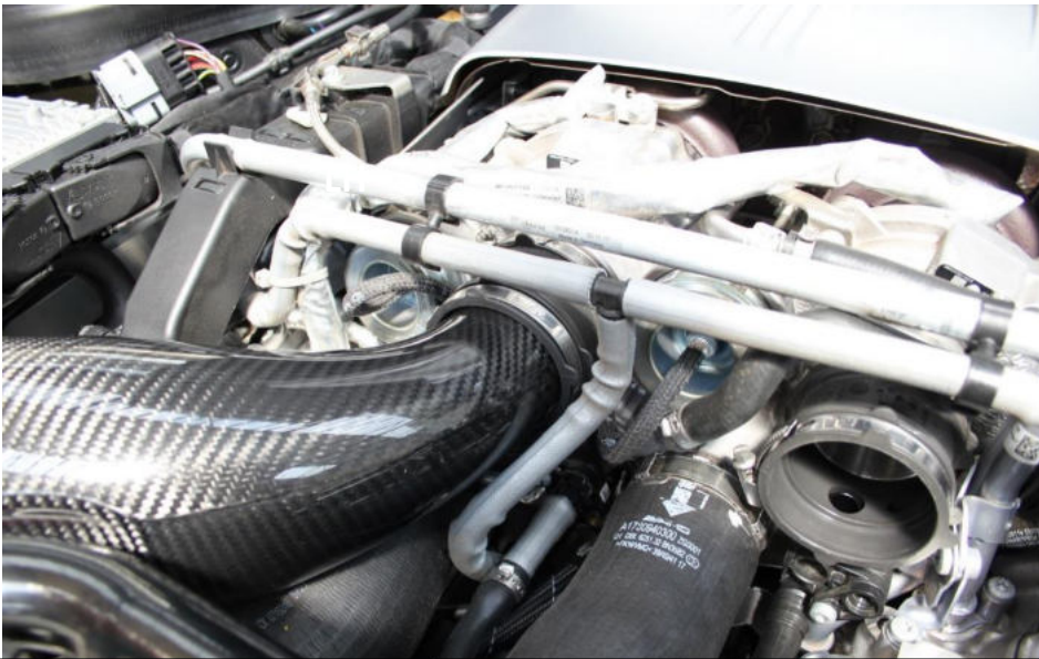
27. Secure the hose clamp at the turbo side – do not over-tighten.
