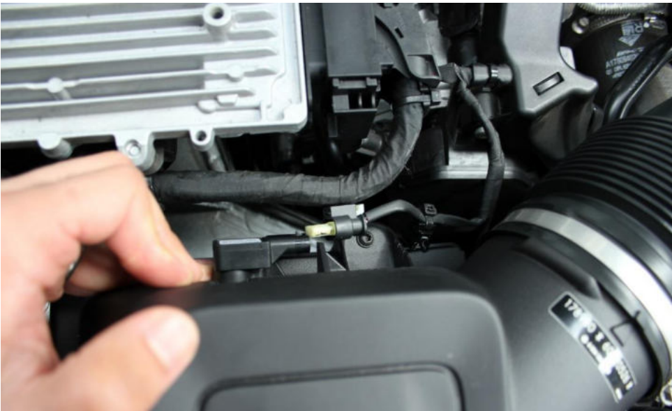
7. Disconnect the MAP sensor at the back of the airbox.
