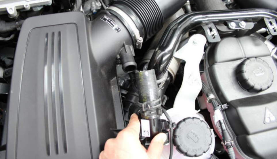
5. Remove the rubber breather hose from the airbox.
