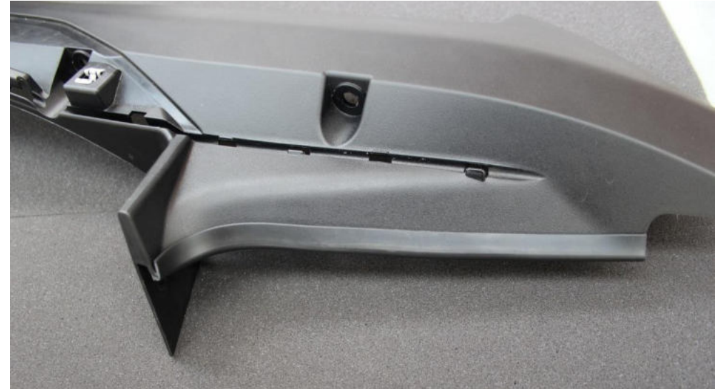
34. Rubber strip in place. Do for both sides.
