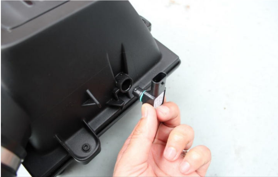
13. Remove the MAP sensors from the airboxes by rotating 90 degrees and pulling out.
