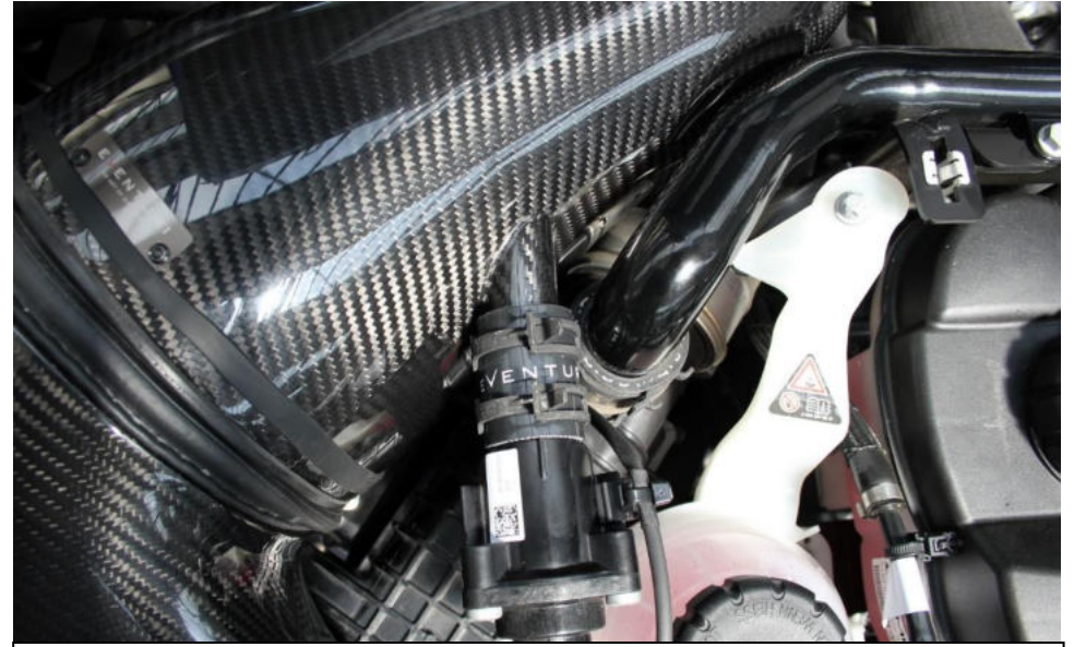
26. Push the silicon tube onto the housing and secure with the clamp.
