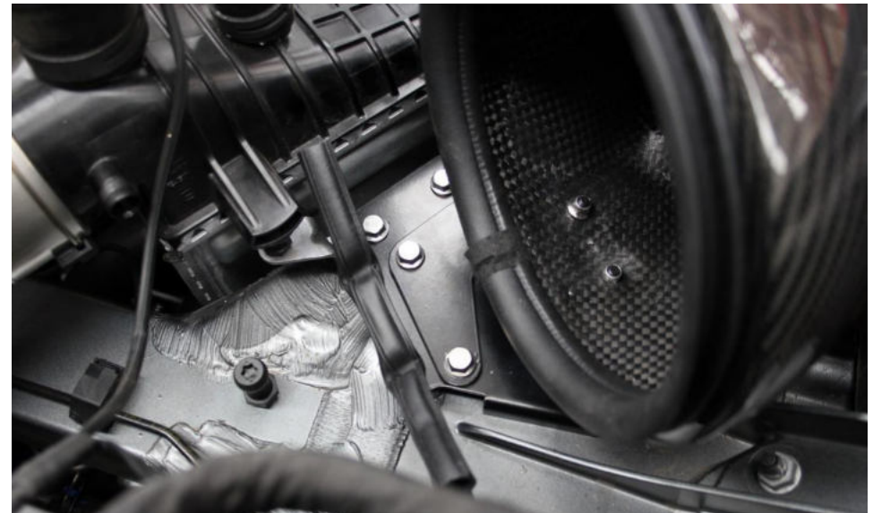
20. Secure the front of the duct onto the base bracket using the 2 M6x12 bolts.
