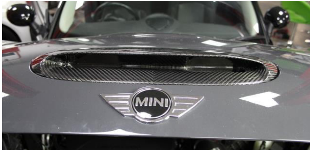
28. Once the clips are in position firmly push the scoop down in all 6 clip positions and ensure they click into place. The clips are firm so please make sure by checking from the underside that they are fully engaged.
