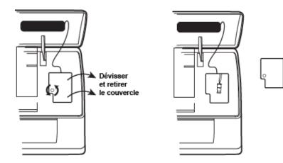
3. Connect the WIFI module connector to the indoor unit WIFI connection cable connector.
