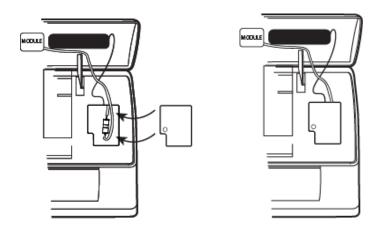
5. Glue the WIFI module to the back of the front panel, next to the black box. An adhesive strip on the back of the module is provided for this purpose.
