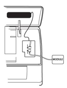
4. Position the module cable upwards. Then close the cover of the electrical connection box using the screw.
