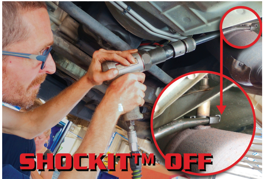
Diesel Tech Kevin Miller uses the 7/8-inch Shockit socket to quickly pull a stuck sensor on a Ford Coyote 5.0L engine.
