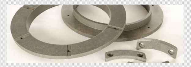
**RAILKO RG2** and **RG12** are based on a woven fabric bonded with resin with the inclusion of a friction modifier. **RAILKO RG2** and **RG12** grades have the advantages of high temperature capability, high compressive strength, high pressure velocity, low friction, and low swell in fluids. The material is used as bushes, bearings, thrust washers, sliding pads.
