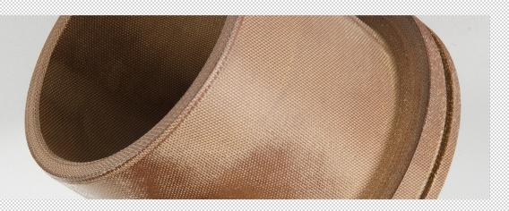
**FEROFORM T814** is a composite material made from woven fibre bonded with resin with PTFE as a friction modifier.
