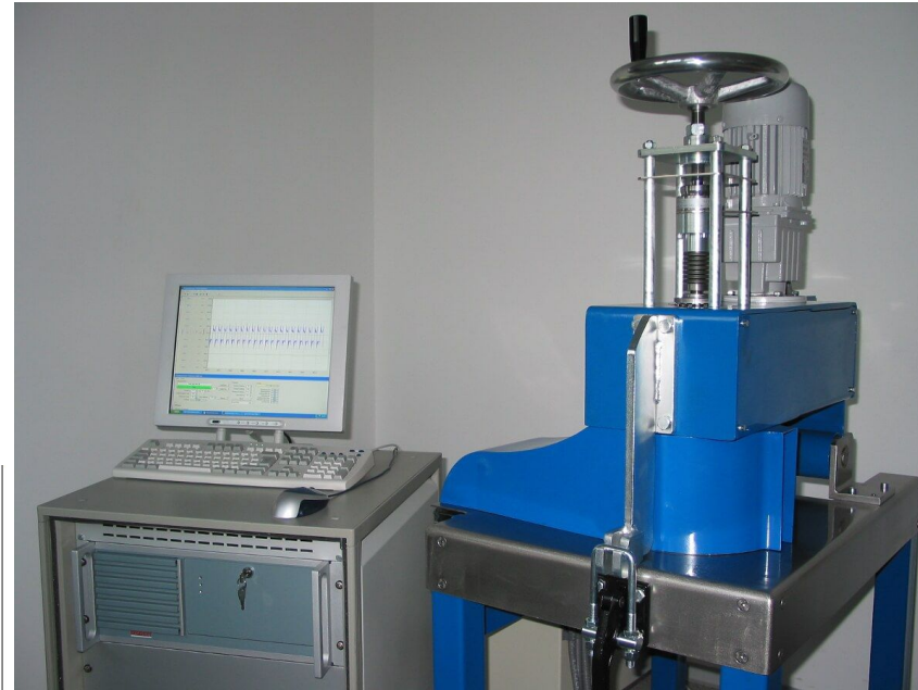
Picture 1: Test equipment to simulate the engine behaviour for friction
