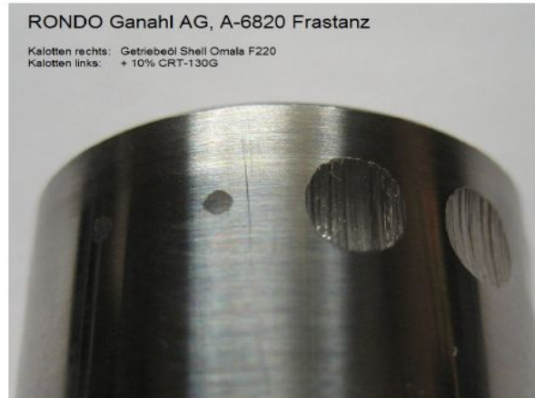
Picture 2: Brugger-Test validation results showing the improved wear situation
