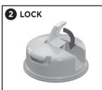
Push down on the suction pad and flip the lever down to lock your suction pad securely in place.\*\*
