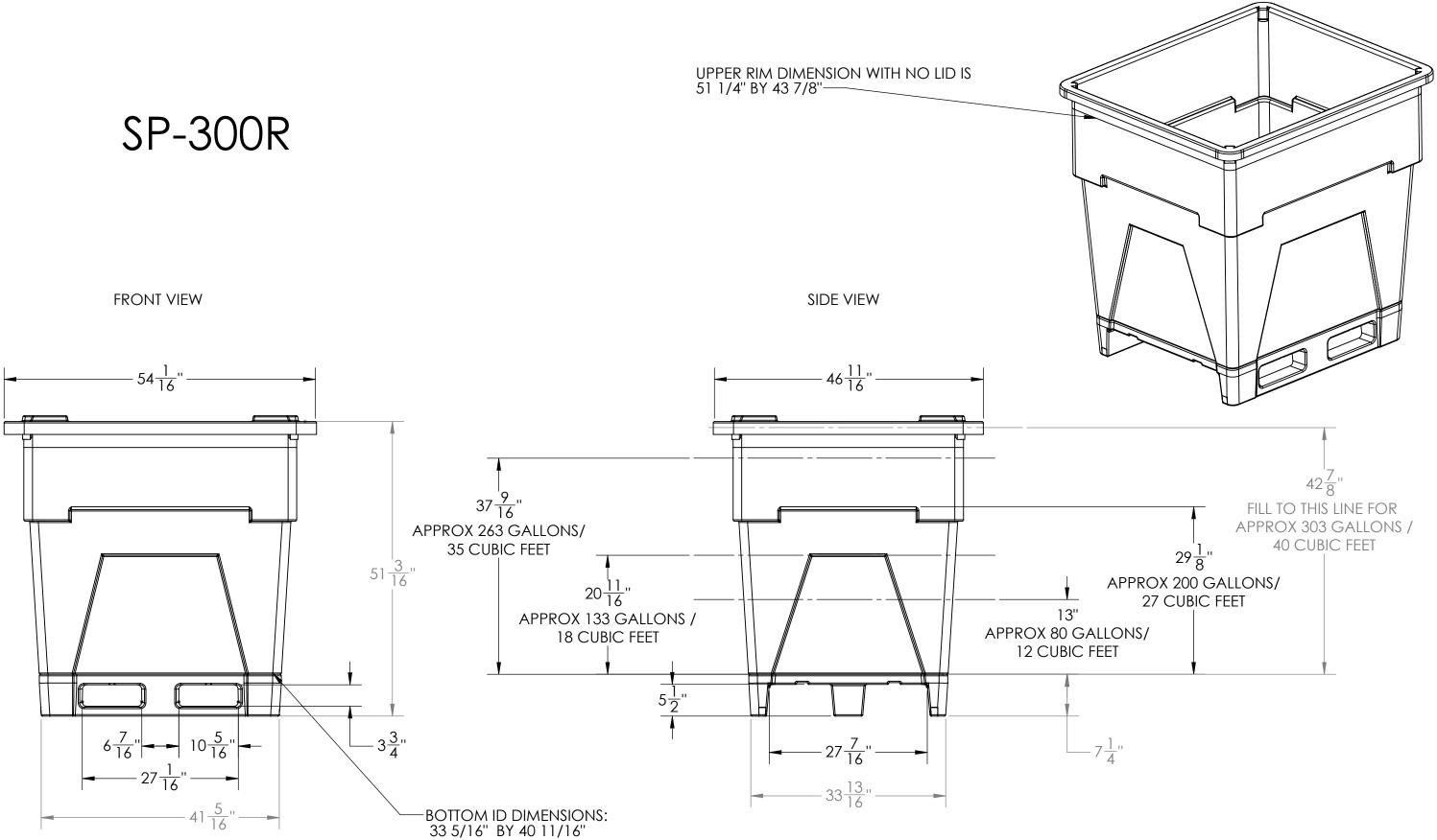
NOTE: 1. CALCULATION ARE BASED OFF OF WATER WEIGHT
