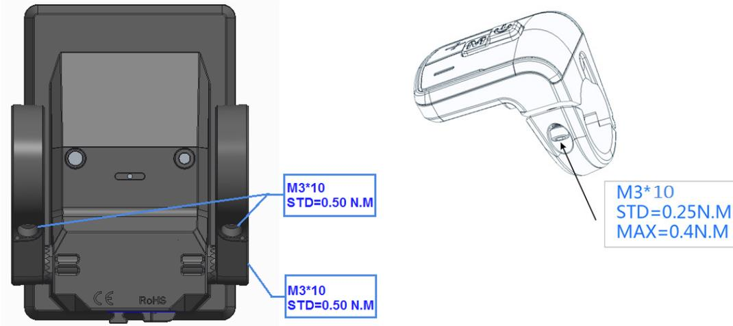
Clamps suit for 3 size of handlebar, 31.8mm, 25.4mm, 22.2mm, there are transfer rings for 25.4mm and 22.2mm, transfer ring must be assembled with the special directions.
