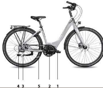
A bicycle drivetrain . The drivetrain consists of the Cranks (1), Chainring (2), Rear Sprocket (4) , Chain (5), Rear Derailleur (3). Bicycle gears are numbered from 1 upwards, with 1 being the lowest and easiest gear.
