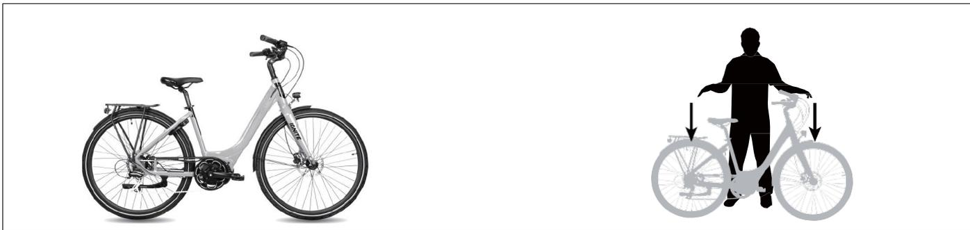
Lift the bike up about 10 cm and drop it to the ground. If you hear any unusual noise or notice issues with Frame stability (especially Frame and Handlepost Joints), book it for a service with your local bike shop.
