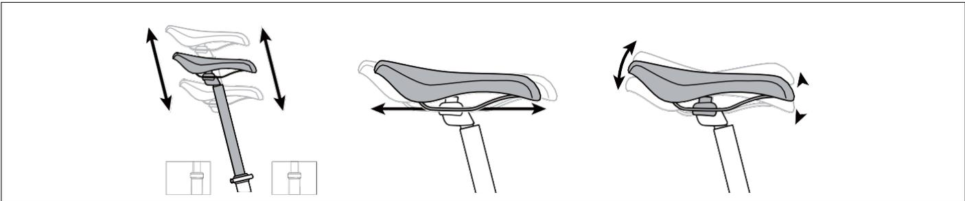
The saddle height is an important component of the overall riding position. While seated, you should have a slight bend in your knee when the Pedal is pushed down all the way. The leg should not be fully extended so make sure the Saddle is not too high. If the seat is too low, repetitive strain on the knee may lead to pain.
