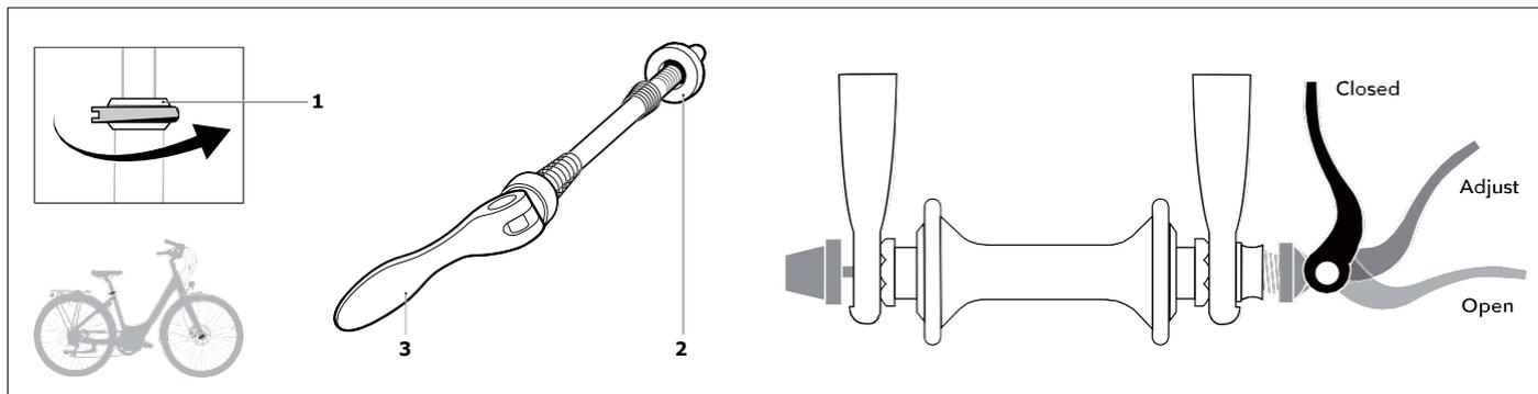
The Quick Release uses over-center cam action to clamp the component in place and allows for easy, tool-less removal.
