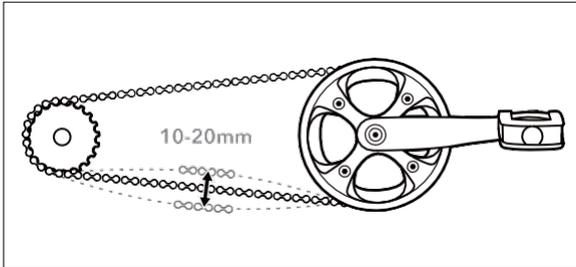
The chain endures huge tension forces from pedaling. For optimal shifting and efficiency, the Chain must connect with the teeth properly.
