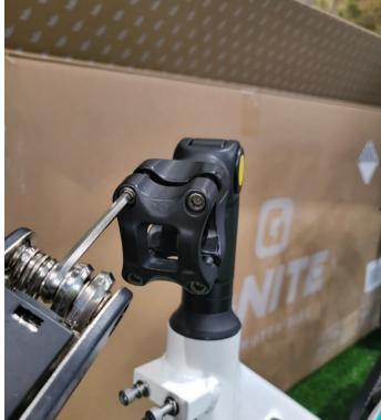
5. Install the handlebars against the stem and then replace the 4 screws to lock in the handlebars.
