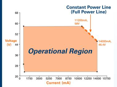
Multiple operating possibilities along the constant power line yields many voltage and current combinations that optimizes the lighting fixture design. Where older designs were limited on the output current due to maximum power constraints, the constant power offerings from MEAN WELL allows for higher current capability.
