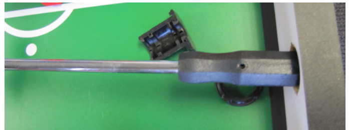
11. Guide handle through opening in near wall in proper position. Pull all the way in to allow other end of rod to clear far wall.
