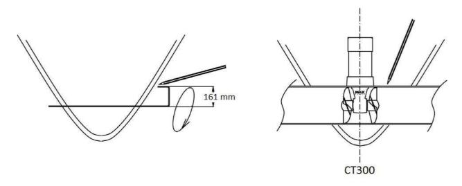
Replace the tunnel. To secure its position apply reinforced fiberglass filler to all areas, both inside and out, taking care to entirely fill the space between the hull and the tunnel. Laminate using a minimum of 8 layers of **ISOPHTALIC RESIN** alternated with mat and roving.
