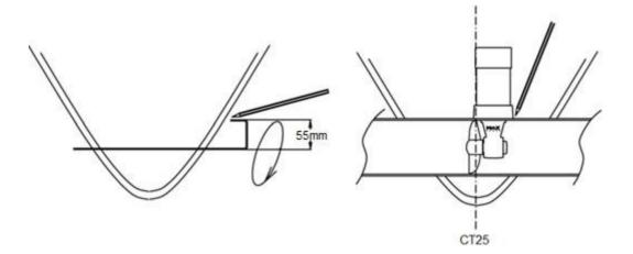
Replace the tunnel. To secure its position apply reinforced fiberglass filler to all areas, both inside and outside, in order to entirely fill the space between the hull and the tunnel. Laminate using a minimum of 8 layers of **ISOPHTALIC RESIN** alternated with mat and roving.
