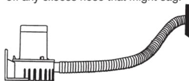
For longer pump life, wire only as directed and **do not run dry**. Turn the switch off immediately after the bilge is pumped.
