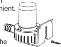
2. Connect the brown wire to the positive (+) lead and switch and connect the black wire to the negative (-) lead. We suggest a 2 A fuse.
