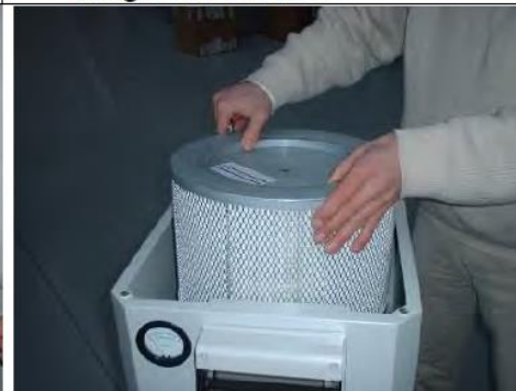
e) Main filter removal
