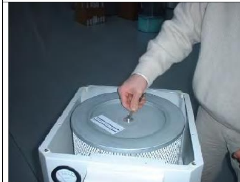
d) Main filter release
