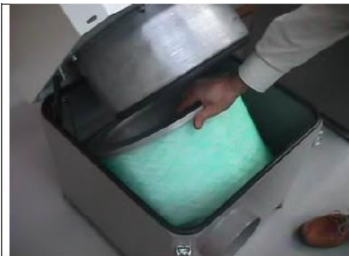
a) Filter re-positioning
