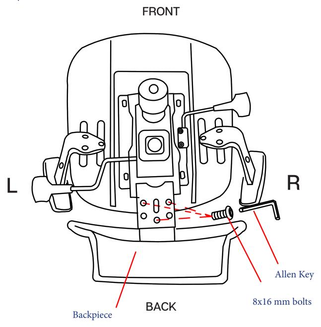
Note: If back piece does not install easily, ensure the metal base is attached on the correct side.
