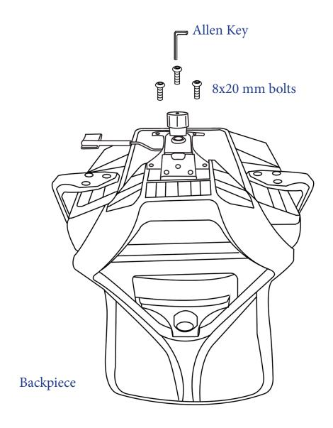
Note: If back piece does not install easily, ensure the metal base is attached on the correct side.
