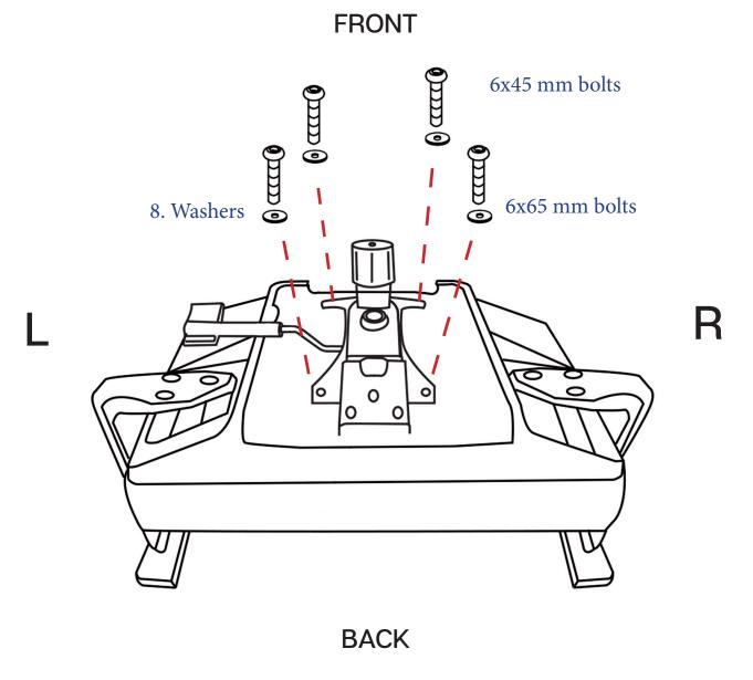
**Note:** The back piece will not connect if the base is installed in the wrong direction.
