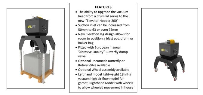
So, you may ask why 2 different types of Hoppers, well first take note of the position of the Forklift Tines and the construction of the leg assemblies. The left-hand photo shows the forklift tines directly under the hopper itself & the leg lock in position is incorporated within the leg itself, the whole assembly is a lighter weight construction designed to be lower in cost & for a broader marketplace such as general factory cleanup of product spills.
