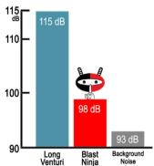
reduces air blast exit velocity while maintaining particle velocity, thus reducing noise while maintaining the abrasive productivity of the nozzle.
