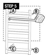
**STEP 5:** Use a tape measure to measure the distance between the center points of each wall bracket tube; record the distances between points AB, AC, CD, and BD. Mounting point C will determine electrical box location. See Electrical Assembly in following instructions.
