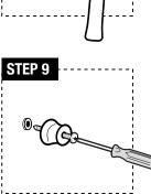
**STEP 9:** Insert long screw (i) through mounting bracket (g), then screw into plastic drywall anchor (f).
