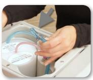
Attach the pink tube from the waste filter to the other end of the short blue tube from the spare parts kit which is already connected to the blue tube coming out of the machine.
