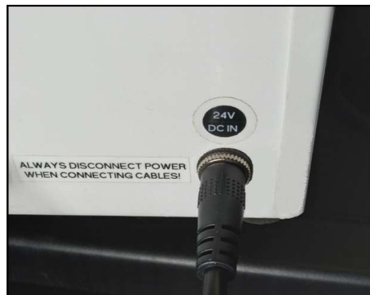
Power adapter to power pack connection
