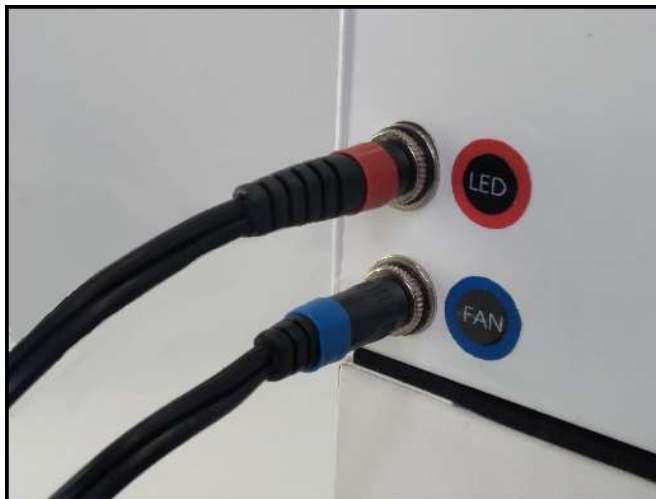
Cable connection to dome assembly
