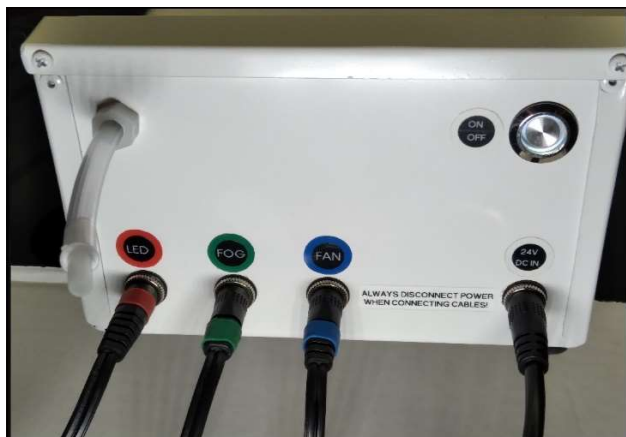
Dome to power pack colored cable connections
