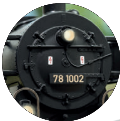
Smoke box door is new, central locking is only present as a dummy
