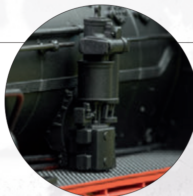
Knorr-Tolkien design feed water pump (with Tolkien control)
