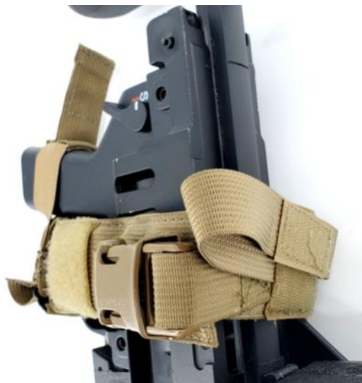
Flat mount 1 inch side-lock buckle was chosen because operators are accustomed to it, and the flat mount gives a stable closure platform. Plastic lined web aligns straps for easy closure.
