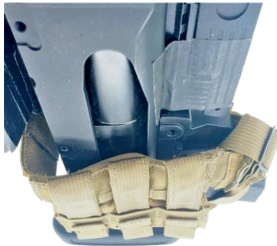
Right handed WRC inverted for wear left handed on left hip. Note clamp indent locks into weapon frame cut-out.
