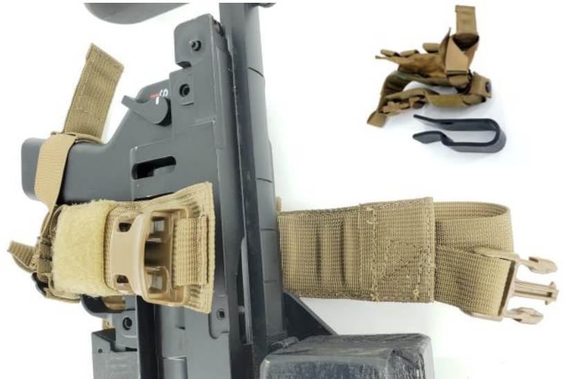
Nylon plastic U-shaped clamp has indent that grasps the M320's frame rather than the trigger guard. Flared at the mouth for quick re-holstering. Plastic lined so it won't dangle and guides buckle. Buckle is angled downward to avoid catching in action if swept inward while re-holstering.
