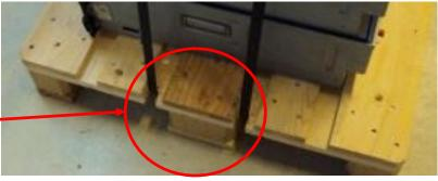
Cut out space for straps on each side of pallet.
