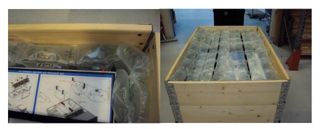
Inside of pallet frame must be fitted with air cushions in all sides and top. (see pictures above).
