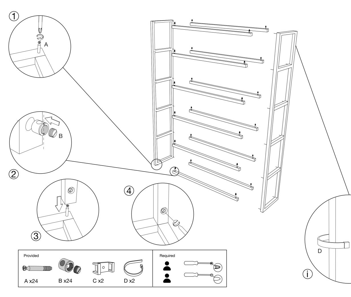
1. Screw threaded pins (A) into all holes in uprights
