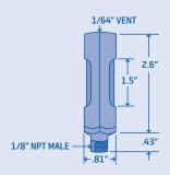
Sights are sized to fit existing or readily available fittings. Heavy duty material is used through (black oxide steel). Sights measure .81" wide by 2.6" high (male) or 2.17" high (female).
