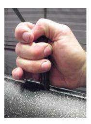
Step 8 - drill one eight hole right 3mm outside of vinyl at each end - DO NOT DRILL VINYL
