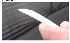
Step 7b - dig point of tool into spline NOT ALL THE WAY THROUGH
