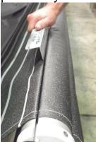
Step 6a - trim end of second spline to aid with insertion
