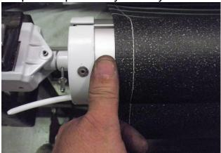
Step 3 - blunt angle tool used to gently press vinyl into second groove - we use 40x40x1.6mm angle that has been smoothed and rounded
