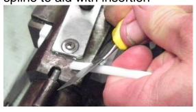
Step 7a - sharp pointed tool to drag spline into second groove
