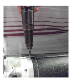
Step 9b - screw should look like this - it stops the vinyl from moving along the roller tube - trim excess spline after screws firmly attached
