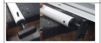
Fit the new pin into the hole and tap into place. It must be visible on both sides of the tube in order to lock the tiller joint into place.
