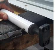
Use a hammer and punch to push the pin out far enough that it can be pulled out with pliers.
