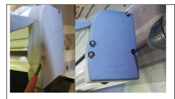
Use a screwdriver to pop out the screw covers and then unscrew the end cap.
