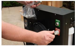
Install the inlet filter onto the inlet connection.
