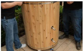
Place the tub back in the desired location with the hose hook ups and the drain facing in the direction required.
