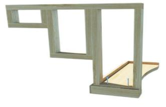
Place the top step of the hot tub steps (curved at the back) upside down and place 1 side of the stairs inside the lip of the side and front of step.
