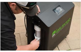
Insert the filter into the holder and screw onto the chiller.
