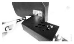
15. Make sure the lighter is burning. Then twist the tap anticlockwise.
