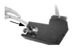
5. Tighten the clamp in clockwise direction.
