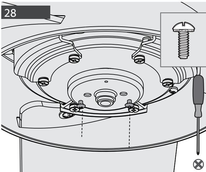
Partially install two light kit assembly screws, found in the ■ hardware bag, halfway into the motor housing as shown. It does not matter which two screw holes you choose.
