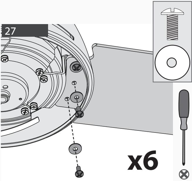
Attach each blade to a blade iron using blade washers, found in the ■ hardware bag, and blade assembly screws, found in the ▲ hardware bag.
