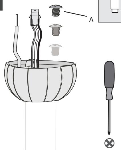
Insert the downrod ball screw (A) into the hole in the top of the downrod ball.
