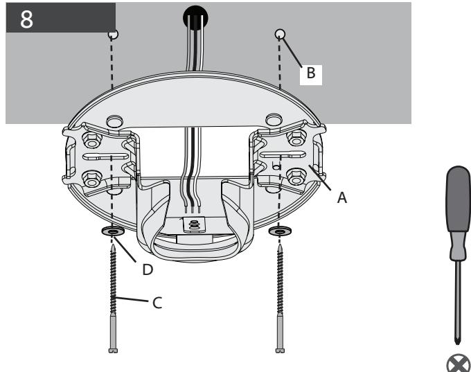
Raise the ceiling plate (A) and align two opposing oval slots with the pilot holes (B). Insert and tighten the two wood screws (C) with washers (D) to secure the ceiling plate (A) to the ceiling.
