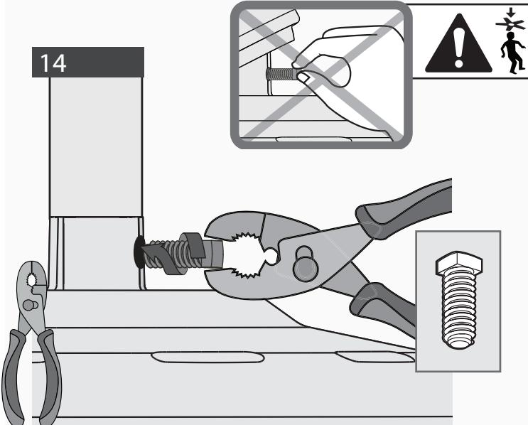
Tighten the setscrew with pliers. **DO NOT HAND TIGHTEN.**
