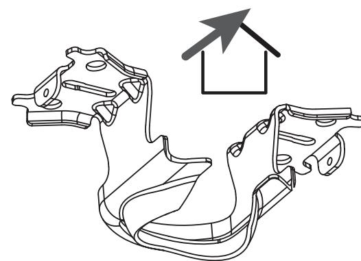
If angle mounting, orient the ceiling plate with the arrows pointing toward the ceiling peak.
