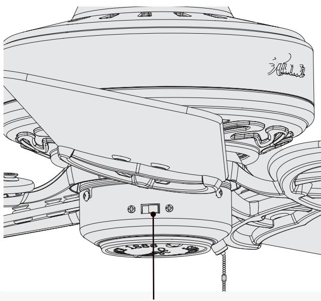
**English** To switch the direction of air flow, move the reverse switch to the opposite position.
