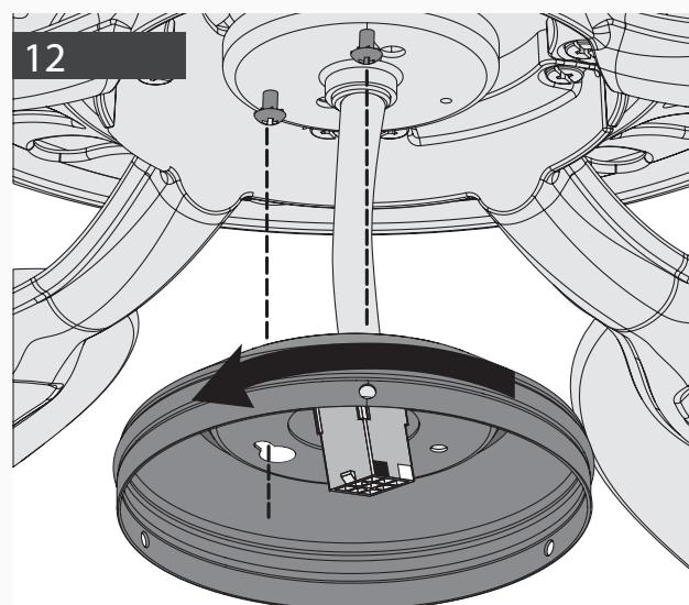
**Feed the wire plug through the center hole of the upper switch housing, then wrap keyhole slots around the screws and twist counterclockwise.**
