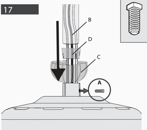
Remove the pre-installed setscrew (A) so that the downrod (B) can be inserted. Save the setscrew (A). Guide the downrod ball (C), sleeve (D), and downrod (B) down the wires coming from the fan.
