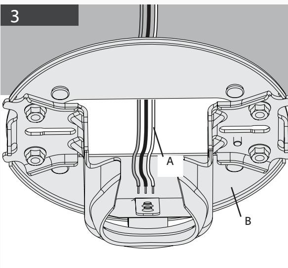
Thread the supply mains (A) through the center hole of the ceiling plate (B).
