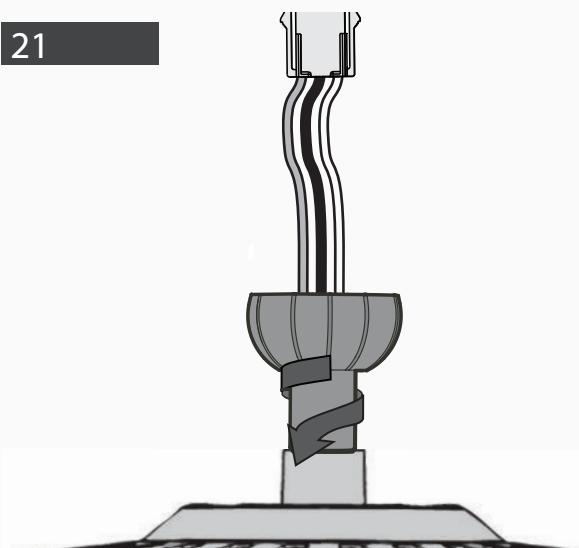
Hand tighten the downrod (at least 4-5 full turns) until it stops.
