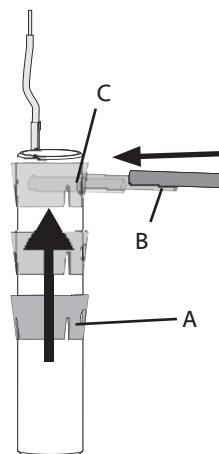
Slide the downrod sleeve (A) up the downrod. Insert the down rod pin (B) into the pin hole (C) on the top of the downrod.
