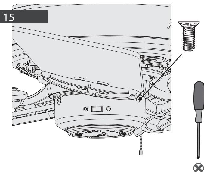
Install the three switch housing screws, found in the hardware bag (Z). Tighten all three screws.
