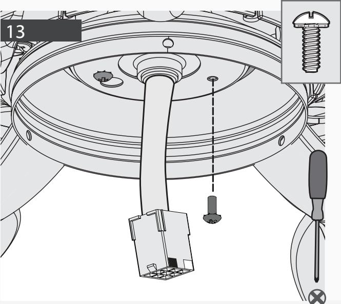
Insert a third light kit assembly screw, found in the hardware bag, into place and tighten all three screws securely.
