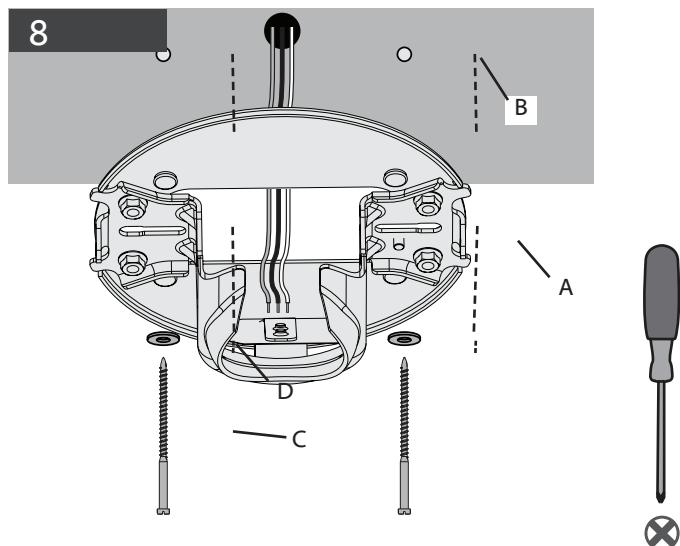
Raise the ceiling plate (A) and align two opposing oval slots with the pilot holes (B). Insert and tighten the two wood screws (C) with washers (D) to secure the ceiling plate (A) to the ceiling.
