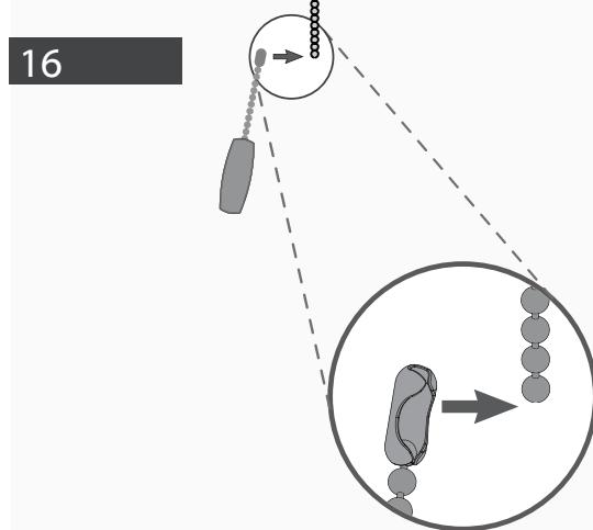
Connect the appropriate pull chain pendant to each of the short chains. The fan pull chain controls the speed: from high to off.
