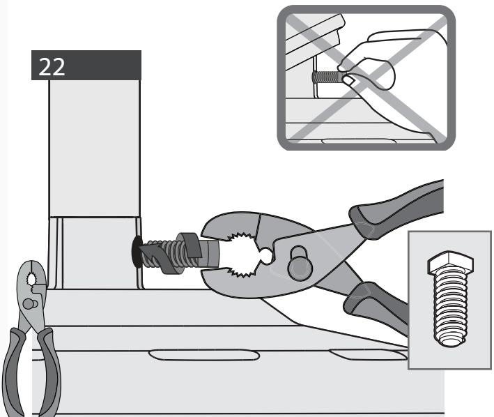
Tighten the setscrew with pliers. **DO NOT HAND TIGHTEN.**
