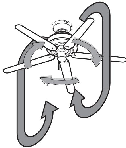
In warm weather, ceiling fans work best by blowing air downward (counterclockwise) providing the room with a cool breeze.
