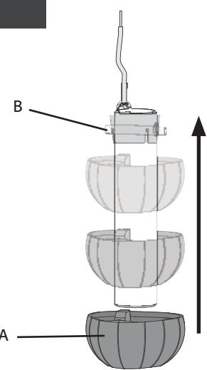
Slide the downrod ball (A) up the length of the downrod pipe. Align the downrod pin (B) with the notches in the downrod ball (A).
