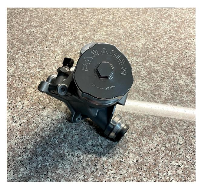
5) With the Engine running inspect the area where the oil filter housing and filter cap meet for any oil leaks, excessive oil loss in this area is likely to occur in the event of improper installation.
