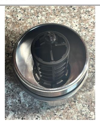
3) With the filter bypass valve transferred to your new cap you may now apply a new O-ring gasket to the exterior of the cap, just as you would with your OEM filter cap.
