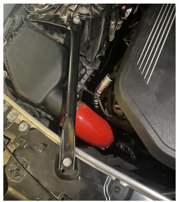
8) Finally with the vehicle on please ensure there are no leaks and that everything has been properly installed. Pictured above is our silicone intake pipe. Our aluminum turbo inlets can be paired with our silicone intake pipes, which will delete all intake resonators entirely, providing smooth unrestricted airflow.
