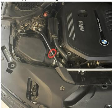
2) Undo all bolts or clips holding the factory airbox together.
