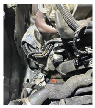
5) Transfer any fittings or clips from the OEM inlet to your new turbo inlet.
