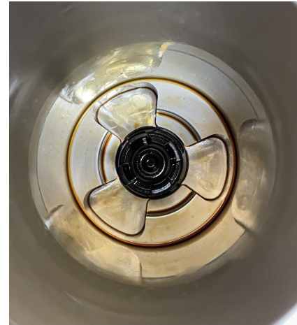
Oil filter cap after installing filter bypass valve.
