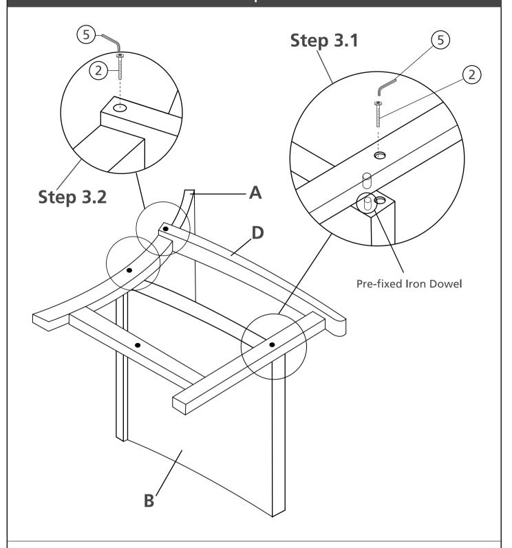
Position housing of Left Leg Panel (D) into pre-fixed iron dowel on Seat Panel (B) as picture
