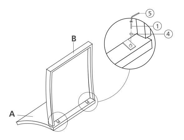
Lay down Backrest Panel (A) then attach Seat Panel (B) to Backrest Panel (A) by using Bolt 1, Flat Washer 4 and secure by Allen Key 5
