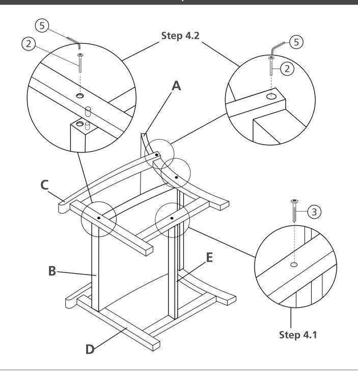
With assistance from your adult partners, turn pre-assemble part in step 3 to the other side Place Leg Support Bar (E) into housing of Left Leg Panel (D) Then, position housing of Right Leg Panel (C) into pre-fixed iron dowel on Seat Panel (B) and Leg Support Bar (E) as picture
