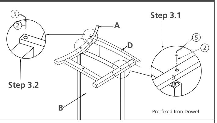
Position housing of Left Leg Panel (D) into pre-fixed iron dowel on Seat Panel (B) as picture
