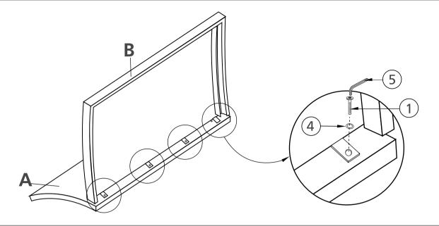
Lay down Backrest Panel (A) then attach Seat Panel (B) to Backrest Panel (A) by using Bolt 1, Flat Washer 4 and secure by Allen Key 5
