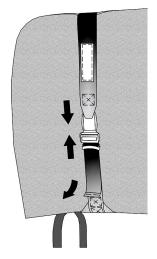
3. Once the crotch strap adjuster is in place, connect the seat belt buckle behind the seat making sure the buckle release is facing toward the seat back. Tighten the webbing until the top of the seat back depresses slightly.
