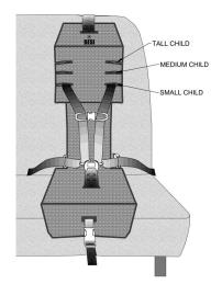
6. Select proper shoulder belt slot for child. Straps should be at or just above the shoulders.
