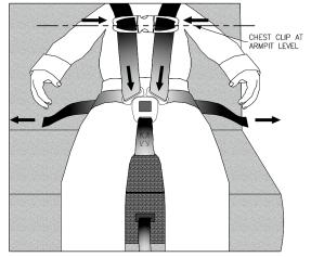
7. Connect child belt buckle and chest clip (adjust to armpit level), then tighten straps by depressing side adjusters and pulling on webbing until snug.
