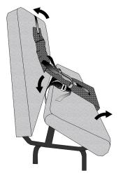
1. Unlatch and tilt seat cushion forward, then slide belt buckle tongue and 1" seat strap between the back and cushion. Re-secure seat cushion to factory specifications. For some seats, you may just need to push the belt buckle and 1" seat strap through the seat bight without lifting seat cushion.
