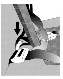
2. Land middle crotch strap adjuster behind Pro Tech seat pad into the seat bight. Crotch strap adjuster should be up high enough to be able to depress the button, but not so high that the student would be sitting on it.
