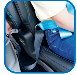
10. Feed bottom tether hook back through bite of seat. Captain's chairs, can go around side of the seat. Repeat step 9-10 for opposite side
