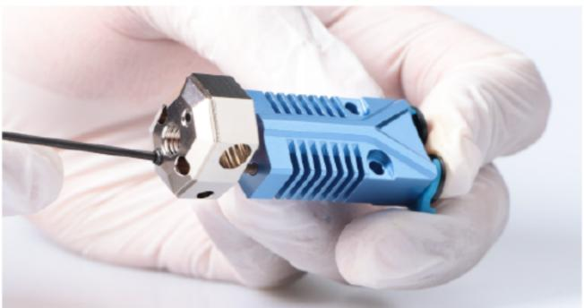
6. Put the silicone sock on the heatblock
