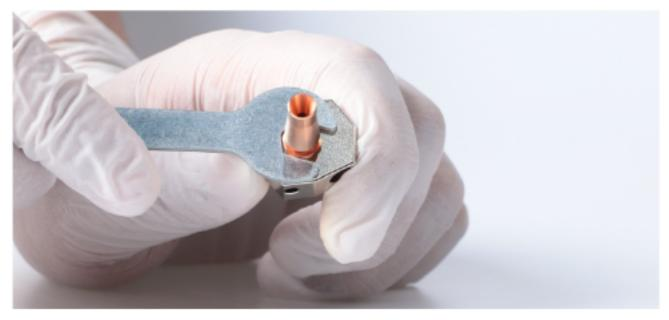
3. Connect the assembled heatblock to the heatsink, and align the two holes on the lower end of the heatsink with the holes on the B side of the heatblock
