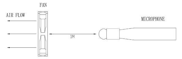
Test Conditions: In the background noise below 17dB (A) noise indoors, vertical rope fastened to the four corners of the fan, put the microphone 1Meter away from the fan centre where air flow input.
