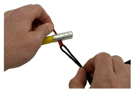
Step 3: With the replacement band's cord captured by the bread tie, thread the bread tie back through the hole on the butt end of the polespear. Pull the bread tie along with the cord all the way through the hole.
