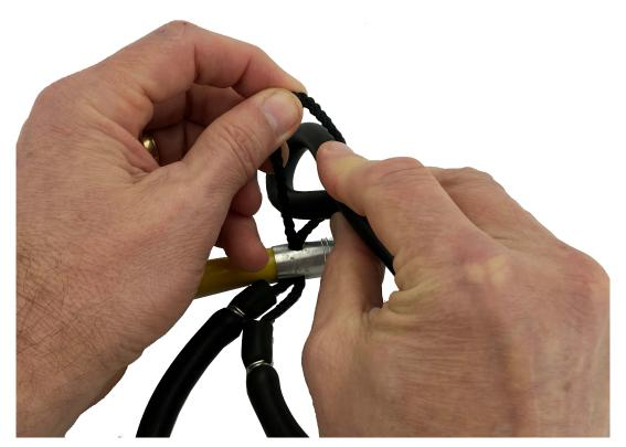
Step 4: With the cord pulled all the way through the hole in the polespear, take the latex band and thread it through the loop on the cord as shown.
