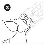
• Hook the band on the bracket bar.
