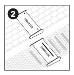
Make sure bracket is positioned between links or locking grooves, then snap bracket into place by pushing down latch.
